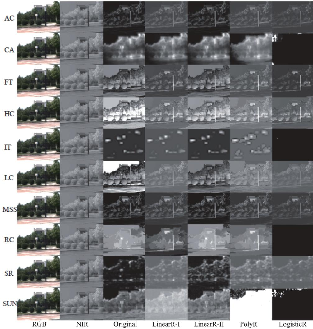
Figure 4: Typical examples of experimental results. The first column to the seventh column respectively represent the RGB image, NIR image, the results using only the original RGB band, the results of combining RGB and NIR bands by LinearR-I, LinearR-II, PolyR and LogisticR models.
