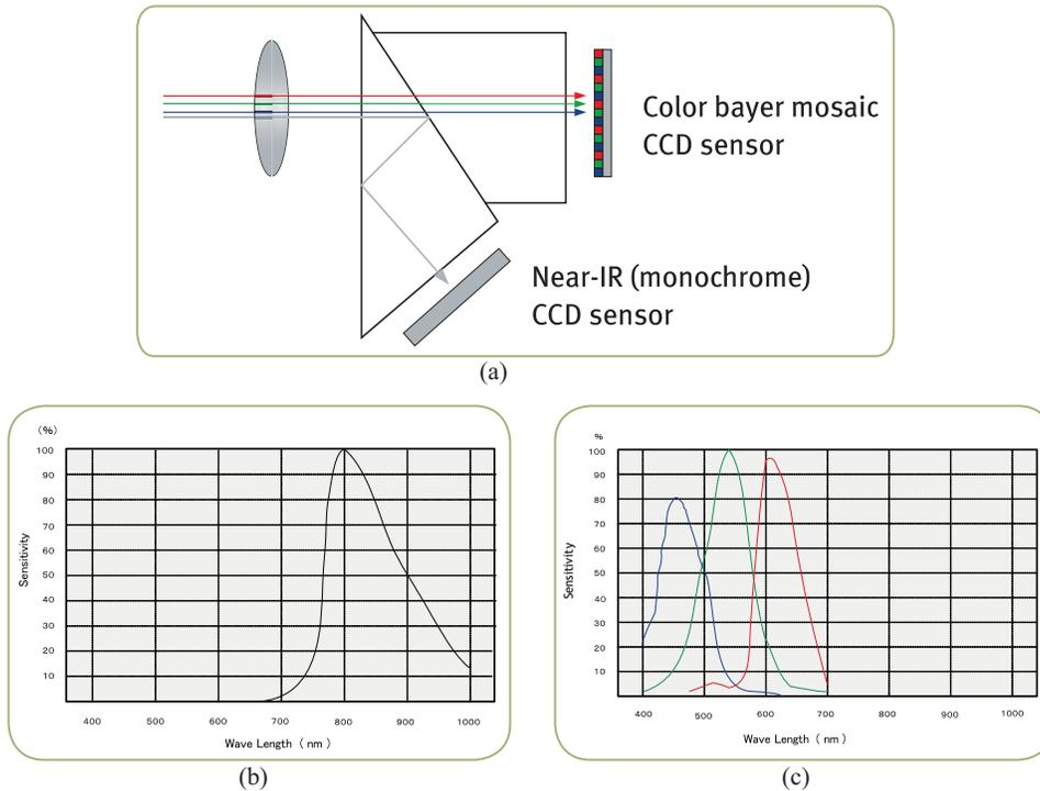
Figure 1: (a) The mechanism of the camera. (b) The CCD response curve to the NIR spectrum. (c) The CCD response curve to the visible light spectrum. These two figures are cited from [28].
